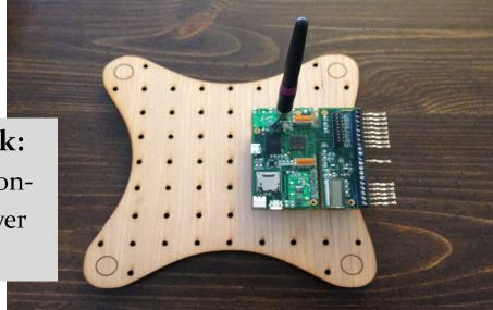
The Micro Framework: with wireless, real-time controller, and advanced power management.
